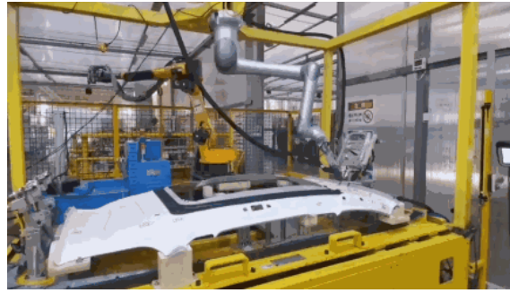
Car roof gluing
