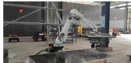
Photovoltaic panel handling
